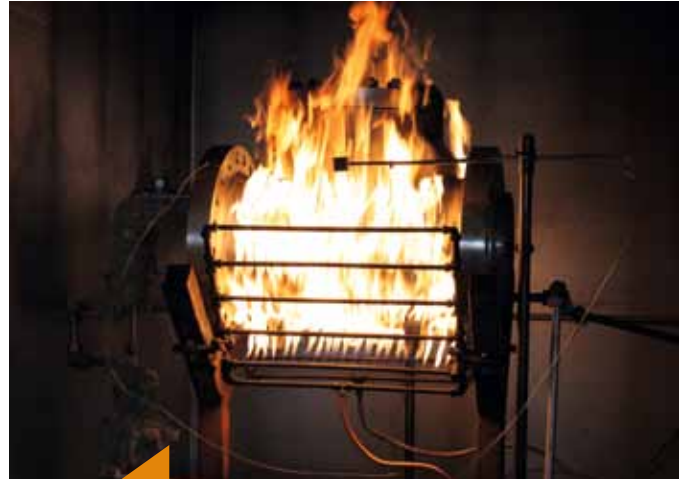
FIRE SAFE TEST OF AN INNO-CHK SWING CHECK VALVE NPS 14 CLASS 600
